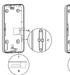
2. Position the mounting plate on a flat surface or wall as to where it will be installed. Mark the 4 holes with a pencil. Drill holes with 6mm (diameter) and 30mm depth.
